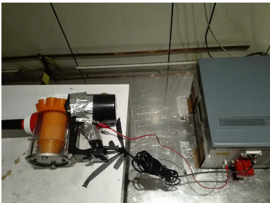
Photograph 2: Set-up for Continuous Disturbance Voltage
